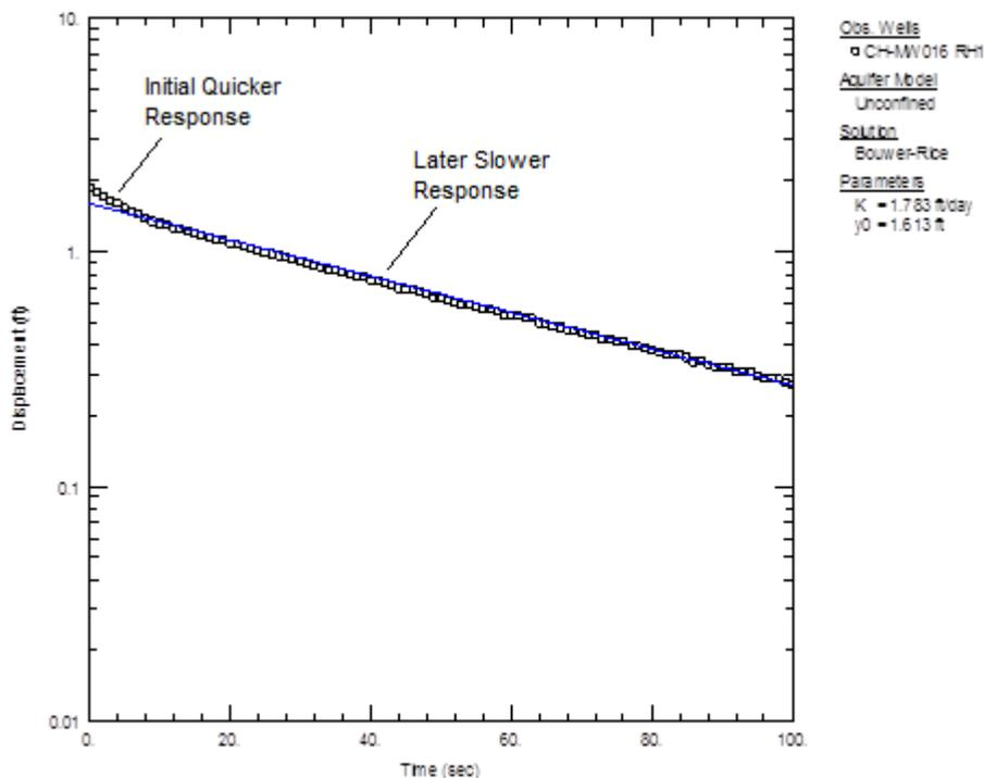
This type of response is known as a double straight line effect and results when filter drainage occurs in a well screened across the water table. The initial quicker response to slug movement is probably due to filter pack drainage, while the slower response that occurs later is more indicative of flow from the aquifer into the well. Analysis of the data from this well focused on the later responses.
