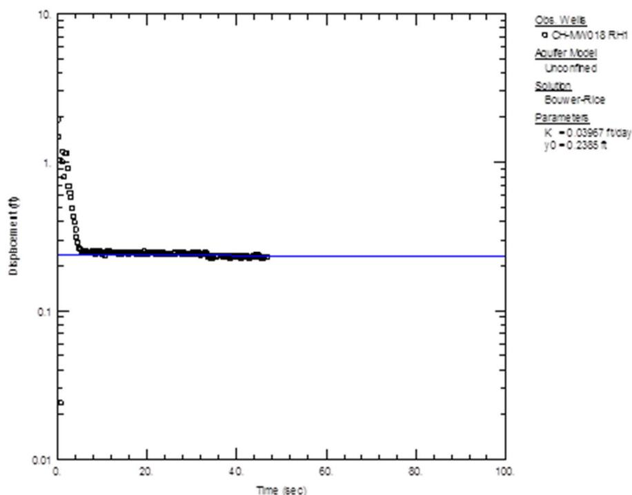
The later slower responses were fit with solutions. The Bouwer-Rice model solution fit the plots of displacement vs. time better than the Hyder et al. (1994) KGS model solution. Estimates of K are representative of glacial till composed primarily of silt at this well location. The results of the Bouwer-Rice model solution are presented in the table below.
